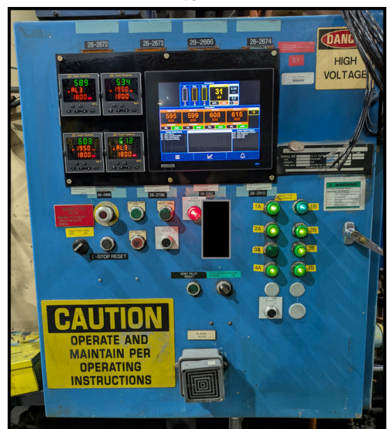
Modern touchscreen interface for temperature and ratio control
